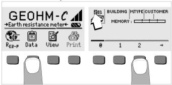
First, enter the desired memory address with the softkeys. After acknowledging this entry with the **START** key (press at center), the cursor appears at the first entry position (BUILDING).
