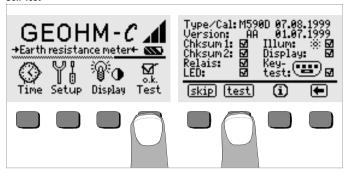
The self-test is started from the main menu with the Test key. The test has a duration of several minutes.
