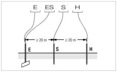
Measuring Earthing Resistance with a 4-Wire Figure 3 Test Setup
