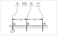
Figure 2 Measuring Earthing Resistance with a 3-Wire Test Setup
