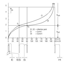
Figure 6 Measuring Earthing Resistance at a Large Earthing System
