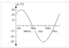
Figure 8 Soil resistivity oE in as influenced by season without taking precipitation into consideration (earth spike depth < 1.5 m)
