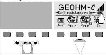
The instrument can be switched on by pressing any key.
