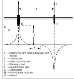
Figure 4 Characteristic Voltage Curve in Homogenous Soil between Earth Electrode E and Auxiliary Earth Electrode H
